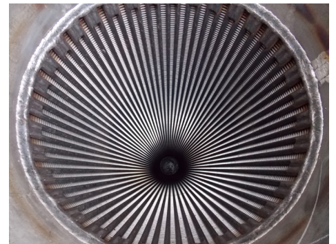
24 in. screen installed
